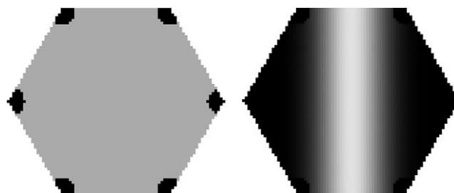
Fig. 4.1. Left: hexagonal simulation domain used in the program HexDiff. The concentration at each corner (black) is fixed to a constant value, due to CF in the apoplastic spaces. Right: CF concentration in the domain immediately following a simulated bleach. Black denotes the highest concentration. The laser passes vertically from the top to the bottom of the domain.
